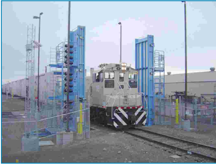
RPMs provide critical protection at rail border crossings, which handle about 70 million metric tons of cargo a year.
