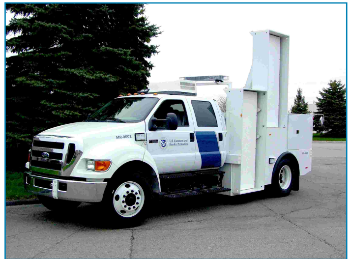
Given the diversity of RPM deployment sites, the RPMP frequently needs to adapt existing technology to meet CBP requirements. Two such adapted systems are the truck-mounted mobile RPM, shown here, and the remotely operated RPM system.
